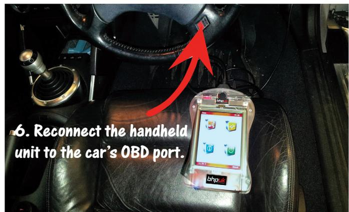
**W**ith ease of use and convenience in mind, BHP's ECU programmer has been designed to read and program vehicle ECUs through the car's diagnostic port – meaning 99% of the time there is no need to dismantle the ECU or remove it from the car.
