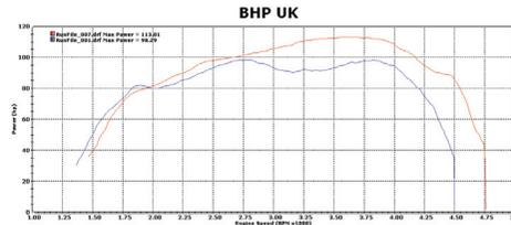
The standard power output (blue) and the smooth version after mapping has taken place (red).
