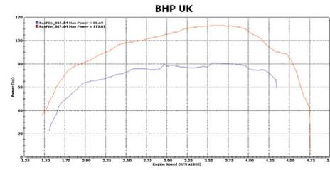
The power output in BHP from the Transit Connect before (blue) and after (red).
